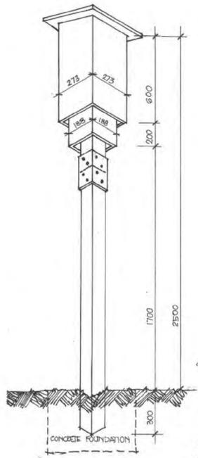
Typical Detail Double Chambered Rocket Box
